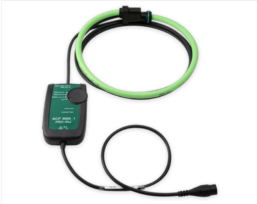
The new PRO-flex ACP 3000\_1 is an AC current probe utilizing the Rogowski principle. It can be used to measure currents up to 3000 A from very low frequencies to 10kHz.
