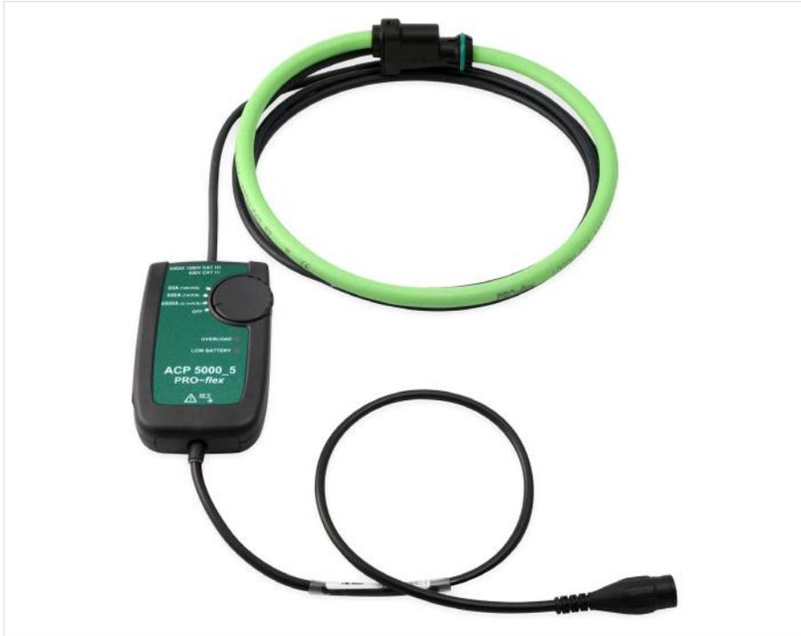
The new PRO-flex ACP 5000\_5 is an AC current probe utilizing the Rogowski principle. It can be used to measure currents up to 5000 A from very low frequencies to 10kHz.
