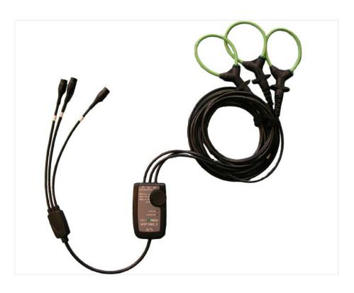
The new Micro-flex ACP 3003\_16 is a 3-Phase AC current clamp utilizing the Rogowski principle. It can be used to measure currents up to 3000A from very low frequencies to 10kHz.
