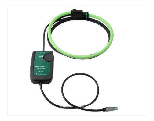
The new PRO-flex ACF 5000 3 is an AC current probe utilizing the Rogowski principle. It can be used to measure currents up to 5000 A from very low frequencies to 10kHz.
