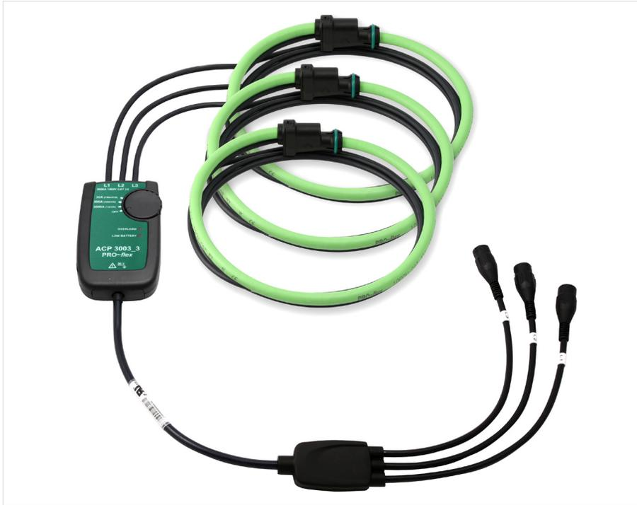
The new PRO-flex ACP 3003\_3 is a 3-Phase AC current probe utilizing the Rogowski principle. It can be used to measure currents up to 3000 A from very low frequencies to 10kHz.
