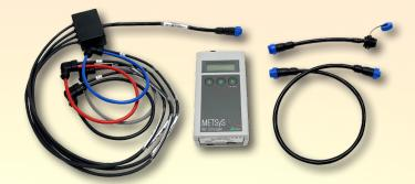
This special accessory package is designed for permanent installation in 480 V cabinets. Included are a 4-phase, 6" diameter MicroFlex current probe assembly rated at 4000A, a thru-panel cabinet adapter/connector and exterior jumper cable to connect the METSyS logger to the cabinet connector plug.
