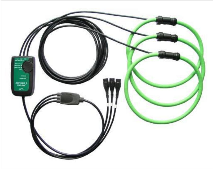
The new PRO-flex ACP 3003\_17 is a 3-Phase AC current probe utilizing the Rogowski principle. It can be used to measure currents up to 3000A from very low frequencies to 10kHz.
