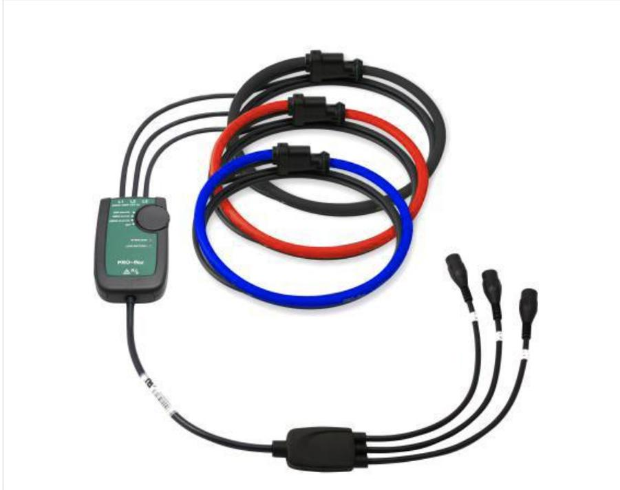
The new PRO-flex ACP 3003\_18 is a 3-Phase AC current probe utilizing the Rogowski principle. It can be used to measure currents up to 3000 A from very low frequencies to 10kHz.
