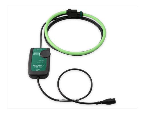
The new PRO-flex ACP 6000 3 is an AC current probe utilizing the Rogowski principle. It can be used to measure currents up to 6000 Amps from very low frequencies to 10kHz.
